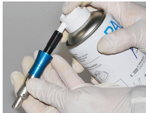
Add about 2–3 puffs into the drive with the oil spray (174010) using the spray nozzle (17401155)
