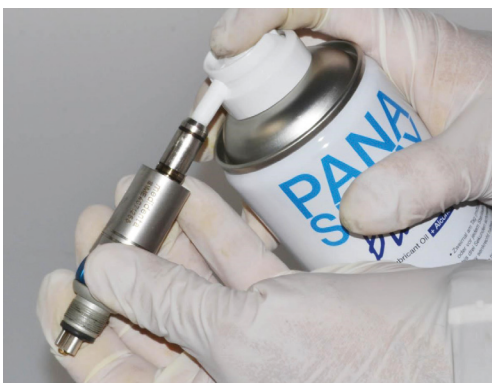
Add about 2–3 puffs into the drift shaft of the turbine with the oil spray (174010) without using the spray nozzle (17401155)
