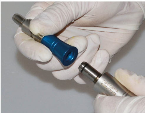
Clean the low speed handpiece externally. Disconnect the low speed handpiece attachment of the turbine.
