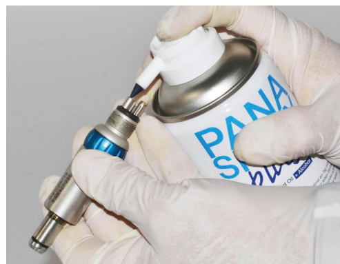
Insert the plug adapter to the oil spray (174010) and spray into the air ducts also two to three times
